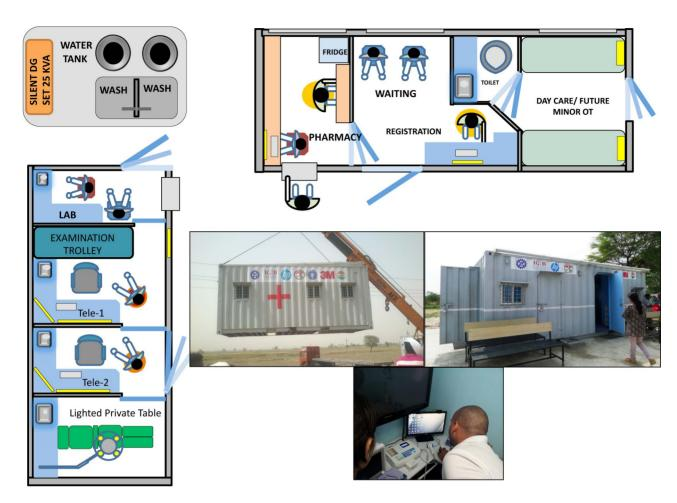
Figure 1. Layout of the eHC. Two  $20 \times 8$  feet containers were used in the proof-of-concept eHC. The telemedicine container (left) has provision for a small laboratory. The second container (top) is used for registration and pharmacy and also has space for a future minor operation theatre. The telemedicine container can be used by itself for basic eHC operations. Pictures of the deployment, exterior, and interior of the telemedicine container are shown.
